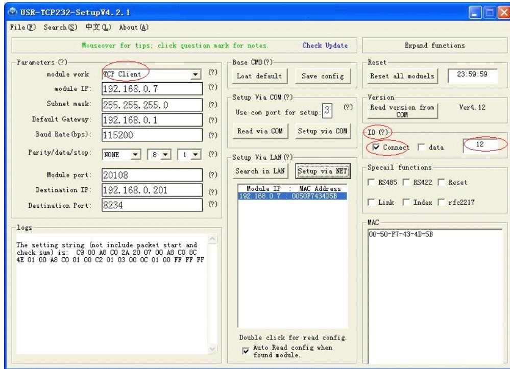
The figure below shows establish a communication connection ID function, the device through the serial communication interface to the TCP Server-side:
