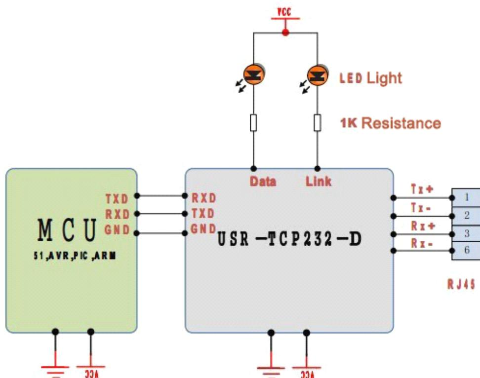
**Note:** Isolation transformer has been on this module, so you need not to add Isolation transformer in your RJ45 port.
