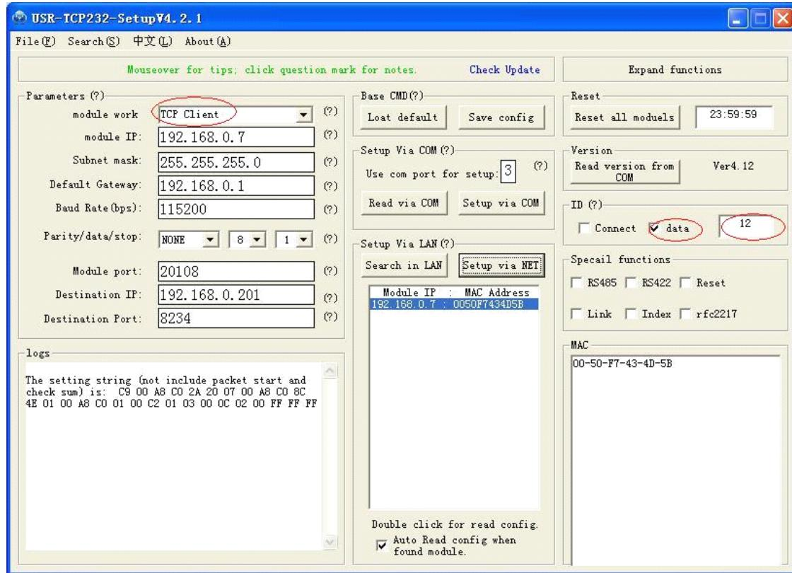
The figure below shows the data communication ID function, the device through the serial port to TCP Server-side communication interface:
