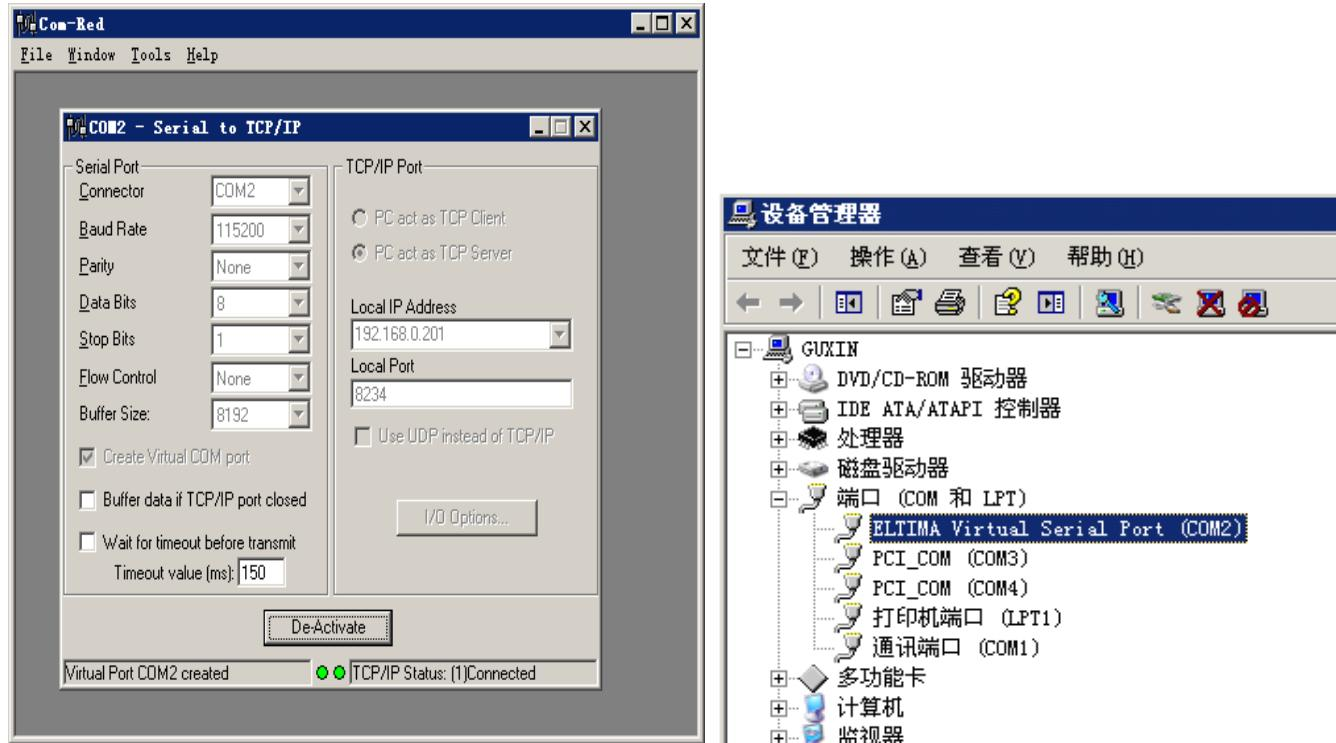
At this point, you can use your equipment as an ordinary serial port, and operate of local virtual serial port will converted to operation of the remote module RS232. The figure is show send data between the two serial port.
