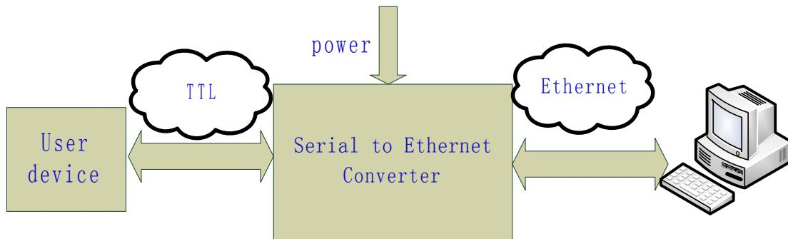
Take USR-TCP232-T for example, show demo application of module USR-TCP232-T
