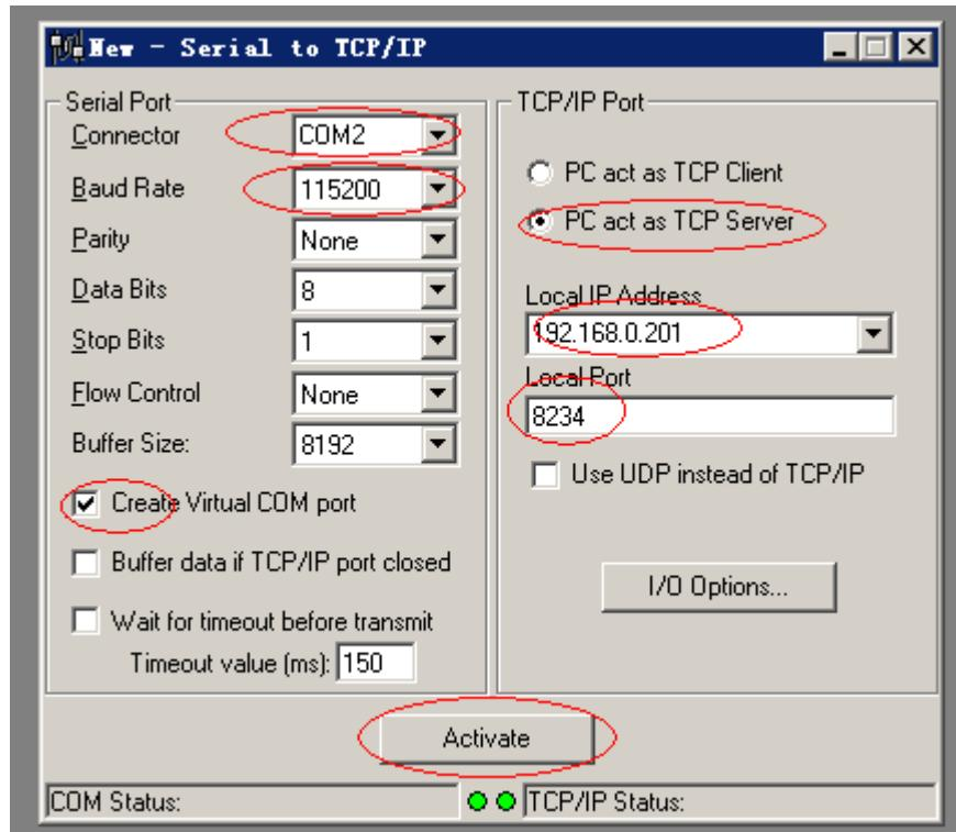
5. After Activate click, a Virtual COM port COM2, will be created, COM2 will receive data from TCPIP socket, and send data to COM2 will convert to TCPIP socket data to remote Equipment.
