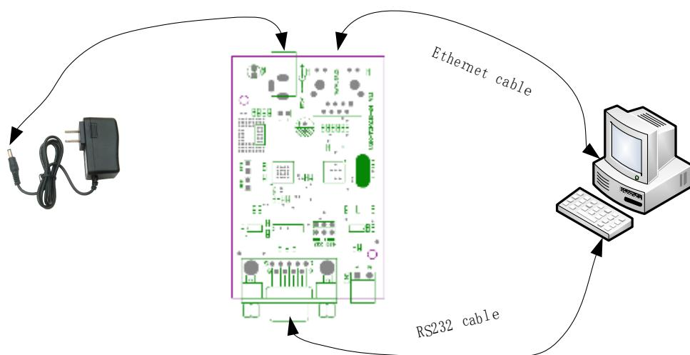
3. Setup the PC's IP address to 192.168.0.201
