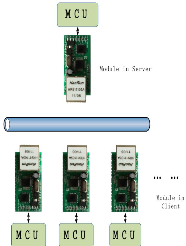
When the UDP server COM transfer data to one of the many COM, the last COM that transferred data will be choose.
