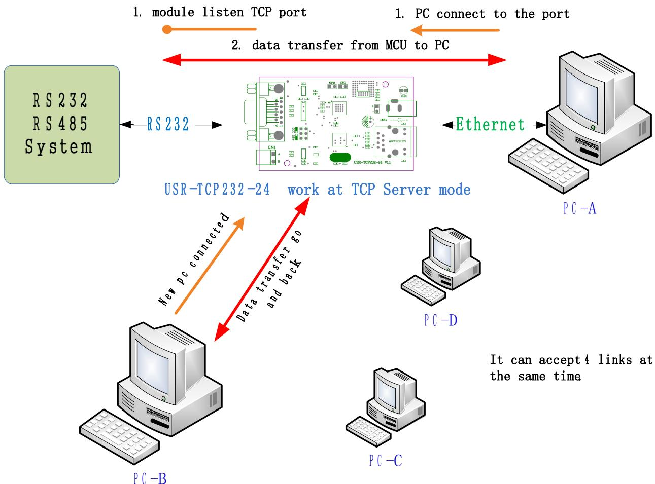
USR-tcp232-24 listen TCP port and accept connect from ethernet.
