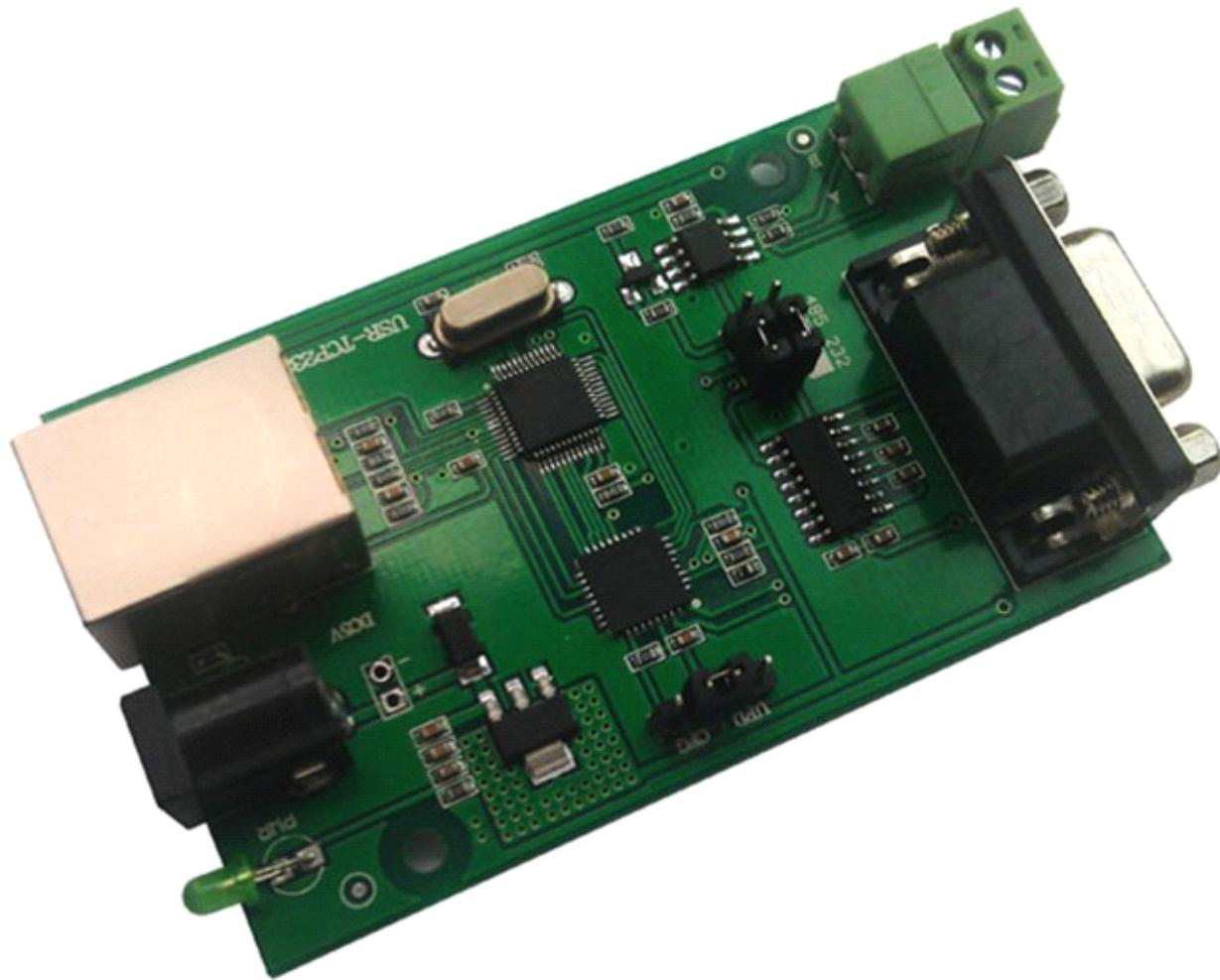
RS232/RS485 to Ethernet convert module is an Equipment for convert TCP or UDP socket data to RS232 or RS485, easy to use, small size, low power, 32 bits arm on board, high speed , high Stability.
